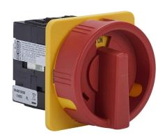
Merz rotary disconnect switch, load break capable, 3-pole, 600 VAC, 32A, 5kA SCCR, door mount, UL 508 rated, front operated. Hardware for 4-hole door mounting & lockable red/yellow handle for use with NEMA 4/4X enclosures included.
