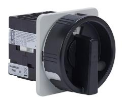
Merz rotary disconnect switch, load break capable, 3-pole, 600 VAC, 32A, 5kA SCCR, door mount, UL 508 rated, front operated. Hardware for 4-hole door mounting & lockable black/gray handle for use with NEMA 4/4X enclosures included.
