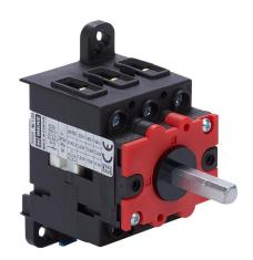
Merz manual motor controller, open, 25A, 600 VAC, 3-pole, 10hp, 35mm DIN rail or panel mount, UL 508 rated.
