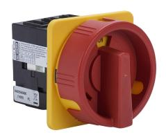
Merz rotary disconnect switch, load break capable, 3-pole, 600 VAC, 25A, 5kA SCCR, door mount, UL 508 rated, front operated. Hardware for 4-hole door mounting & lockable red/yellow handle for use with NEMA 4/4X enclosures included.
