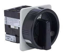
Merz rotary disconnect switch, load break capable, 3-pole, 600 VAC, 25A, 5kA SCCR, door mount, UL 508 rated, front operated. Hardware for 4-hole door mounting & lockable black/gray handle for use with NEMA 4/4X enclosures included.
