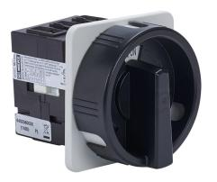
Merz rotary disconnect switch, load break capable, 3-pole, 600 VAC, 25A, 5kA SCCR, door mount, UL 508 rated, front operated. Hardware for 4-hole door mounting & lockable black/ gray handle for use with NEMA 4/4X enclosures included.
