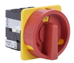
Merz rotary disconnect switch, load break capable, 3-pole, 600 VAC, 16A, 5kA SCCR, door mount, UL 508 rated, front operated. Hardware for 4-hole door mounting & lockable red/yellow handle for use with NEMA 4/4X enclosures included.
