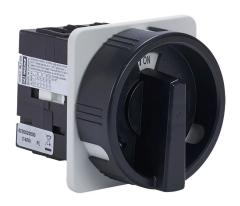
Merz rotary disconnect switch, load break capable, 3-pole, 600 VAC, 16A, 5kA SCCR, door mount, UL 508 rated, front operated. Hardware for 4-hole door mounting & lockable black/gray handle for use with NEMA 4/4X enclosures included.
