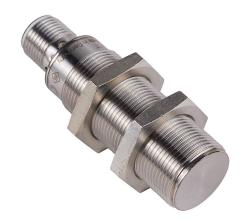
AutomationDirect magnetic proximity sensor, tubular, 18mm diameter x 60mm body, 316L stainless steel housing, PNP, N.C. output, 70mm sensing distance, flush, 5 kHz switching frequency, IP65 IP67, 4-pin M12 quick-disconnect.
