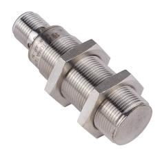
AutomationDirect magnetic proximity sensor, tubular, 18mm diameter x 60mm body, 316L stainless steel housing, PNP, N.O. output, 70mm sensing distance, flush, 5 kHz switching frequency, IP65 IP67, 4-pin M12 quick-disconnect.
