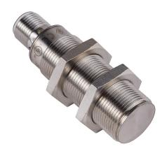
AutomationDirect magnetic proximity sensor, tubular, 18mm diameter x 60mm body, 316L stainless steel housing, NPN, N.O. output, 70mm sensing distance, flush, 5 kHz switching frequency, IP65 IP67, 4-pin M12 quick-disconnect.
