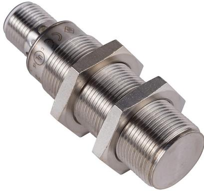
AutomationDirect magnetic proximity sensor, tubular, 18mm diameter x 60mm body, 316L stainless steel housing, NPN, N.O. output, 70mm sensing distance, flush, 5 kHz switching frequency, IP65 IP67, 4-pin M12 quick-disconnect.
