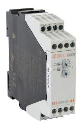
Dold off-delay relay timer, 0.05 seconds to 300 hours selectable timing range, 12-240 VAC/VDC operating voltage, 3A contact rating, (1) DPDT timed relay output(s), 35mm DIN rail mount, screw terminal(s).
