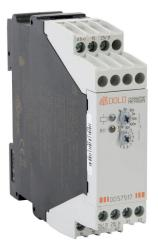
Dold on-delay relay timer, 0.05 seconds to 300 hours selectable timing range, 12-240 VAC/VDC operating voltage, 3A contact rating, (1) SPDT timed relay and (1) SPDT instant or timed configured relay output(s), 35mm DIN rail mount, screw terminal(s).
