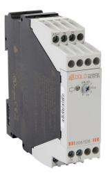
Dold off-delay relay timer, 0.15 to 3 seconds timing range, 24-240 VAC/VDC operating voltage, 3A contact rating, (1) DPDT timed relay output(s), 35mm DIN rail mount, screw terminal(s).
