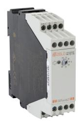
Dold off-delay relay timer, 1.5 to 30 seconds timing range, 24-240 VAC/VDC operating voltage, 3A contact rating, (1) DPDT timed relay output(s), 35mm DIN rail mount, screw terminal(s).
