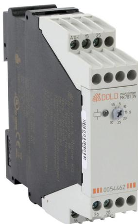
Dold off-delay relay timer, 1.5 to 30 seconds timing range, 24-240 VAC/VDC operating voltage, 3A contact rating, (1) DPDT timed relay output(s), 35mm DIN rail mount, screw terminal(s).
