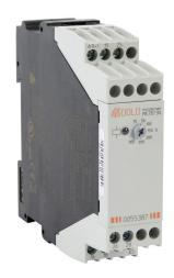
Dold off-delay relay timer, 15 to 300 seconds timing range, 24-240 VAC/VDC operating voltage, 3A contact rating, (1) DPDT timed relay output(s), 35mm DIN rail mount, screw terminal(s).
