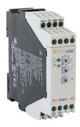
Dold multi-mode relay timer, 0.02 seconds to 300 hours selectable timing range, 12-240 VAC/VDC operating voltage, 3A contact rating, (1) SPDT timed relay and (1) SPDT instant or timed configured relay output(s), 35mm DIN rail mount, screw terminal(s).
