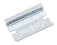
Fibox DIN rail, unslotted, 35 mm width, 7 mm height, 1.97in length, galvanized steel. Package of 1. For use with ULPCM100xxx MNX series enclosures.
