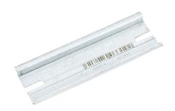
Fibox DIN rail, unslotted, 35 mm width, 7 mm height, 3.94in length, galvanized steel. Package of 1. For use with ULPCM100xxx ULPCM125xxx and ULPCM150xxxMNX series enclosures.
