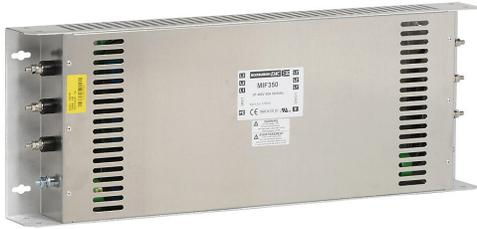
Roxburgh EMI input filter, 230/460 VAC, 3-phase, 50A, panel mount, EMI/RFI filtering, multi-stage, drive rated, very high performance, studs. For use with 3-phase AC drives.
