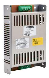
Roxburgh EMI input filter, 120/240 VAC, 1-phase, 10A, panel mount, EMI/RFI filtering, multi-stage, drive rated, very high performance, screw terminals. For use with 1-phase AC drives.
