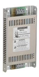
Roxburgh EMI input filter, 120/240 VAC, 1-phase, 3A, panel mount, EMI/RFI filtering, multi-stage, drive rated, very high performance, spring clamp terminals. For use with 1-phase AC drives.
