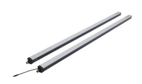
ReeR Micron light grid, sender/receiver pair, measuring, 30mm resolution, 870mm detection height, 0-10m operating distance, (2) push-pull, (2) 4-20mA analog output, configurable, (1) 5-pin M12 quick-disconnect and (1) 8-pin M12 quick-disconnect.
