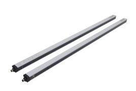
ReeR Micron light grid, sender/receiver pair, measuring, 10mm resolution, 890mm detection height, 0-10m operating distance, PNP, configurable, (2) 5-pin M12 quick-disconnects, IO-Link compatible.
