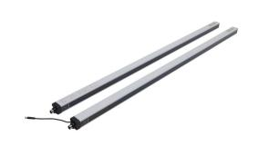
ReeR Micron light grid, sender/receiver pair, measuring, 10mm resolution, 890mm detection height, 0-10m operating distance, (2) push-pull, (2) 4-20mA analog output, configurable, (1) 5-pin M12 quick-disconnect and (1) 8-pin M12 quick-disconnect.
