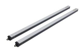
ReeR Micron light grid, sender/receiver pair, object detection, 30mm resolution, 720mm detection height, 0-10m operating distance, (2) push-pull complementary, (2) 5-pin M12 quick-disconnects.
