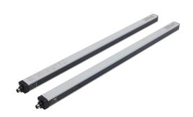
ReeR Micron light grid, sender/receiver pair, measuring, 30mm resolution, 570mm detection height, 0-10m operating distance, PNP, configurable, (2) 5-pin M12 quick-disconnects, IO-Link compatible.
