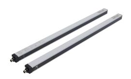
ReeR Micron light grid, sender/receiver pair, measuring, 10mm resolution, 590mm detection height, 0-10m operating distance, PNP, configurable, (2) 5-pin M12 quick-disconnects, IO-Link compatible.
