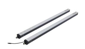
ReeR Micron light grid, sender/receiver pair, measuring, 10mm resolution, 590mm detection height, 0-10m operating distance, (2) push-pull, (2) 4-20mA analog output, configurable, (1) 5-pin M12 quick-disconnect and (1) 8-pin M12 quick-disconnect.
