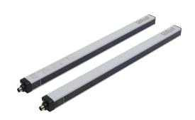
ReeR Micron light grid, sender/receiver pair, object detection, 30mm resolution, 420mm detection height, 0-10m operating distance, (2) push-pull complementary, (2) 5-pin M12 quick-disconnects.
