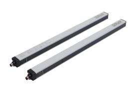
ReeR Micron light grid, sender/receiver pair, object detection, 10mm resolution, 440mm detection height, 0-10m operating distance, (2) push-pull complementary, (2) 5-pin M12 quickdisconnects.
