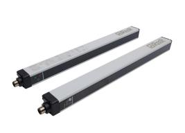
ReeR Micron light grid, sender/receiver pair, measuring, 30mm resolution, 270mm detection height, 0-10m operating distance, PNP, configurable, (2) 5-pin M12 quick-disconnects, IO-Link compatible.
