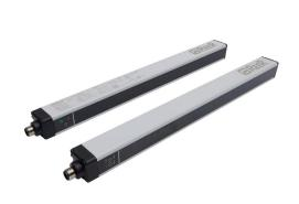
ReeR Micron light grid, sender/receiver pair, object detection, 30mm resolution, 270mm detection height, 0-10m operating distance, (2) push-pull complementary, (2) 5-pin M12 quick-disconnects.
