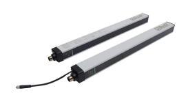
ReeR Micron light grid, sender/receiver pair, measuring, 30mm resolution, 270mm detection height, 0-10m operating distance, (2) push-pull, (2) 4-20mA analog output, configurable, (1) 5-pin M12 quick-disconnect and (1) 8-pin M12 quick-disconnect.
