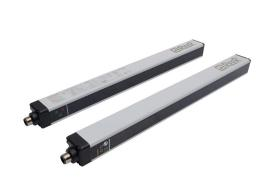
ReeR Micron light grid, sender/receiver pair, measuring, 10mm resolution, 290mm detection height, 0-10m operating distance, PNP, configurable, (2) 5-pin M12 quick-disconnects, IO-Link compatible.
