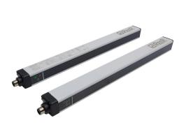
ReeR Micron light grid, sender/receiver pair, object detection, 10mm resolution, 290mm detection height, 0-10m operating distance, (2) push-pull complementary, (2) 5-pin M12 quickdisconnects.
