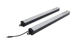
ReeR Micron light grid, sender/receiver pair, measuring, 10mm resolution, 290mm detection height, 0-10m operating distance, (2) push-pull, (2) 4-20mA analog output, configurable, (1) 5-pin M12 quick-disconnect and (1) 8-pin M12 quick-disconnect.
