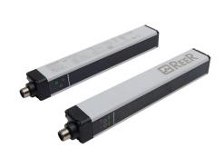
ReeR Micron light grid, sender/receiver pair, object detection, 30mm resolution, 120mm detection height, 0-10m operating distance, (2) push-pull complementary, (2) 5-pin M12 quick-disconnects.
