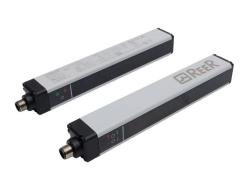
ReeR Micron light grid, sender/receiver pair, object detection, 10mm resolution, 140mm detection height, 0-10m operating distance, (2) push-pull complementary, (2) 5-pin M12 quickdisconnects.
