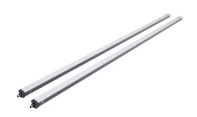
ReeR Micron light grid, sender/receiver pair, measuring, 30mm resolution, 1470mm detection height, 0-10m operating distance, PNP, configurable, (2) 5-pin M12 quick-disconnects, IO-Link compatible.
