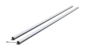
ReeR Micron light grid, sender/receiver pair, measuring, 30mm resolution, 1470mm detection height, 0-10m operating distance, (2) push-pull, (2) 4-20mA analog output, configurable, (1) 5-pin M12 quick-disconnect and (1) 8-pin M12 quick-disconnect.
