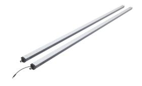
ReeR Micron light grid, sender/receiver pair, measuring, 10mm resolution, 1490mm detection height, 0-10m operating distance, (2) push-pull, (2) 4-20mA analog output, configurable, (1) 5-pin M12 quick-disconnect and (1) 8-pin M12 quick-disconnect.
