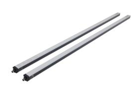
ReeR Micron light grid, sender/receiver pair, measuring, 30mm resolution, 1170mm detection height, 0-10m operating distance, PNP, configurable, (2) 5-pin M12 quick-disconnects, IO-Link compatible.
