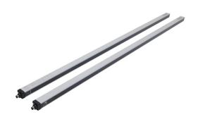
ReeR Micron light grid, sender/receiver pair, measuring, 30mm resolution, 1170mm detection height, 0-10m operating distance, PNP, configurable, (2) 5-pin M12 quick-disconnects, IO-Link compatible.
