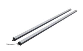
ReeR Micron light grid, sender/receiver pair, measuring, 30mm resolution, 1170mm detection height, 0-10m operating distance, (2) push-pull, (2) 4-20mA analog output, configurable, (1) 5-pin M12 quick-disconnect and (1) 8-pin M12 quick-disconnect.
