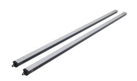
ReeR Micron light grid, sender/receiver pair, measuring, 10mm resolution, 1190mm detection height, 0-10m operating distance, PNP, configurable, (2) 5-pin M12 quick-disconnects, IO-Link compatible.
