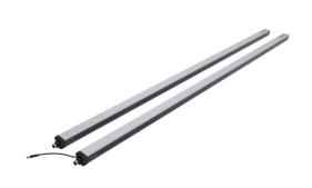
ReeR Micron light grid, sender/receiver pair, measuring, 10mm resolution, 1190mm detection height, 0-10m operating distance, (2) push-pull, (2) 4-20mA analog output, configurable, (1) 5-pin M12 quick-disconnect and (1) 8-pin M12 quick-disconnect.
