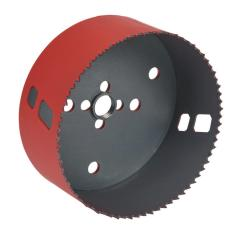
MK Morse hole saw, 4-3/4in (121mm), bi-metal cobalt, hardened steel backer, varied tooth, 1-15/16in (50mm) maximum cutting depth.
