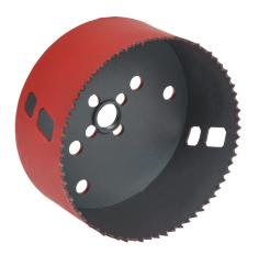
MK Morse hole saw, 4-1/2in (114mm), bi-metal cobalt, hardened steel backer, varied tooth, 1-15/16in (50mm) maximum cutting depth.
