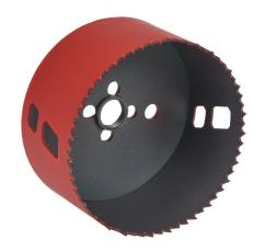
MK Morse hole saw, 4in (102mm), bi-metal cobalt, hardened steel backer, varied tooth, 1-15/16in (50mm) maximum cutting depth.
