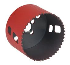
MK Morse hole saw, 3in (76mm), bi-metal cobalt, hardened steel backer, varied tooth, 1-15/16in (50mm) maximum cutting depth.
