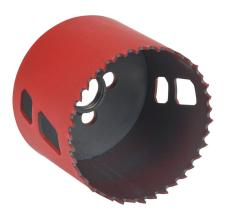
MK Morse hole saw, 2-5/8in (67mm), bi-metal cobalt, hardened steel backer, varied tooth, 1-15/16in (50mm) maximum cutting depth.
